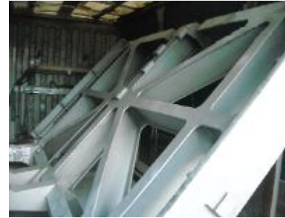
Airbus wing forming tooling: 4m X 3m (1,1 Tn)
