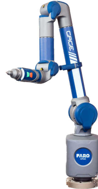
3D Arm Measurement (FARO arm) with laser device for Casting.
